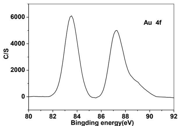
Figure 3 The narrow XPS spectra of the Au 4f region for MWCNTs-gold nanoparticles.
