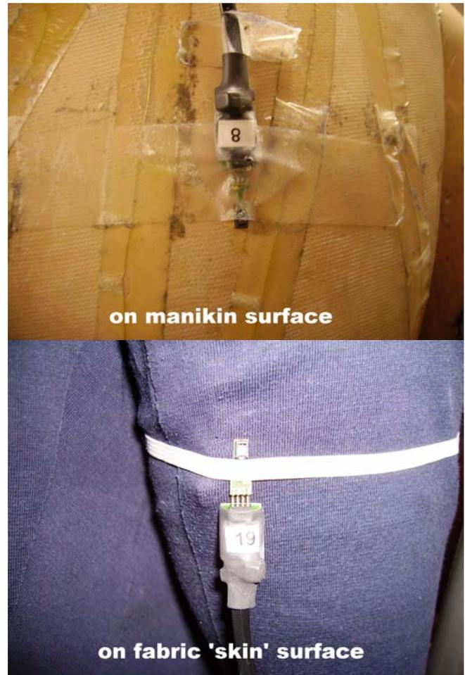
Figure 2 Sensor attachments applied in the study.
