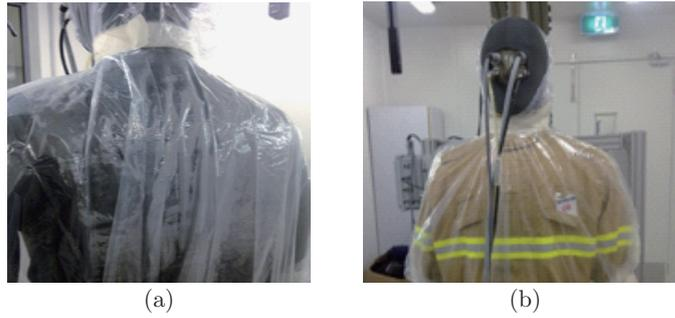
Fig. 2: Thermal manikin clothed with: (a) cooling vest and PVC membrane (A), and (b) firefighter's ensemble and PVC membrane (B)
