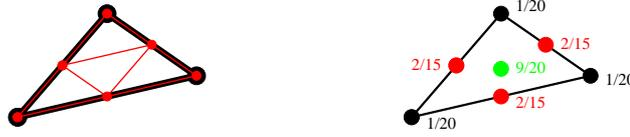
Figure 3: Left: Refinement scheme: each triangle (thick black points and lines), is subdivided into 4 smaller triangles (thin red points and lines). Right: Quadrature rules on each triangle. The quadrature weights in units of the area of the triangle are shown for each node.
